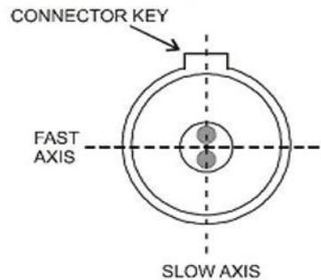
The output light is polarized along the slow axis of PM fiber.
