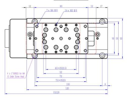
Recommended Mounting Condition: 5um flatness in 120x60 area, 3.2N-m tightening torque on M4X16.
