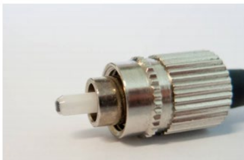
SAM chip on FC/PC connector end face
