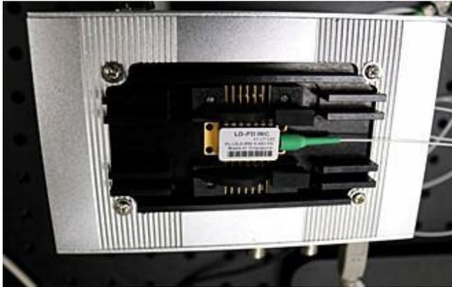
488nm PMFP Laser diode
